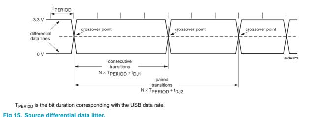
Fig 15. Source differential data jitter.
